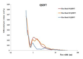
Fig. 3. Pore size distribution for samples S9, S10, S3.
