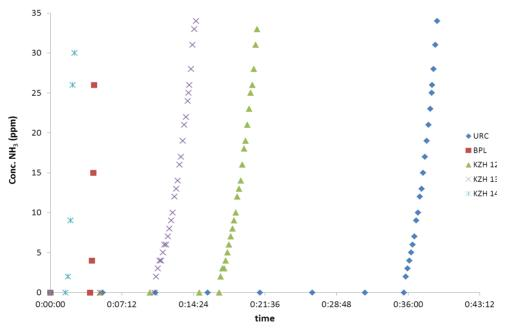
Fig. 6. Experimental breakthrough curves (NH<sub>2</sub>).
