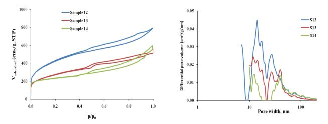
Fig. 4. Low-temperature nitrogen adsorption isotherms and pore size distribution for samples S12, S13, S14.
