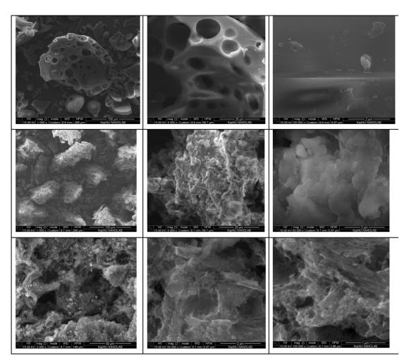
Fig. 1. Electron micrographs and geometry of the binder material – lignosulfonate and the granules obtained on the ground of RH and LS prior to and following carbonization.
