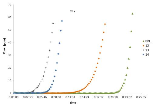
Fig. 5. Experimental curves of cyclohexane breakthrough time using different samples of an amount of 20 g.
