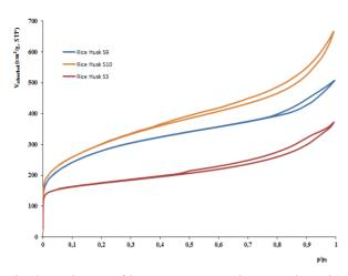
Fig. 2. Isotherms of low-temperature nitrogen adsorption on the samples studied.
