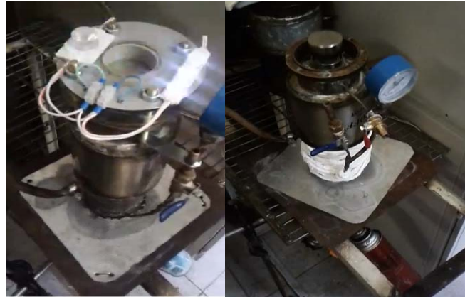
Figure 3 – Experimental laboratory installation with a capacity of 100 W
