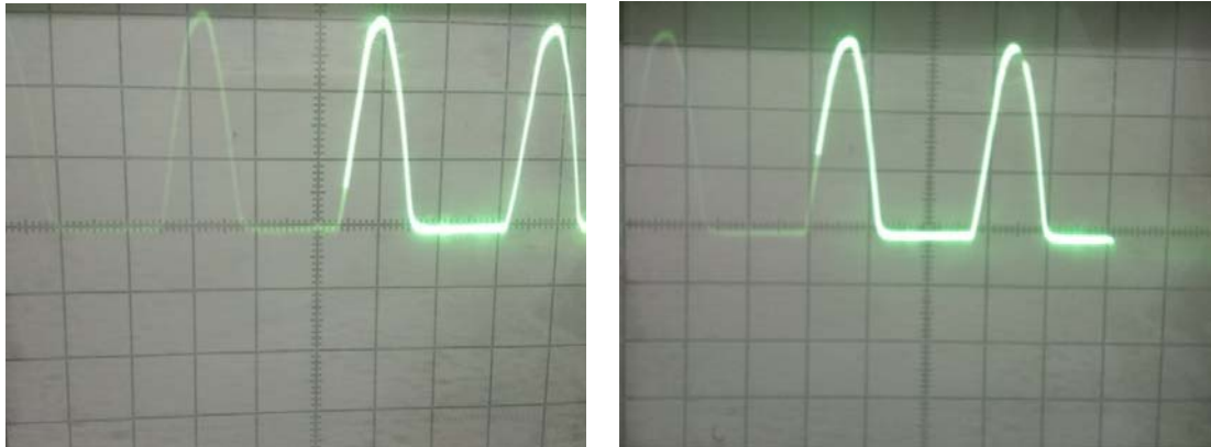
Figure 2 – Oscillogram of the amplitude of the current passing through each circuit of the electrolyzer when polarized with alternating current
